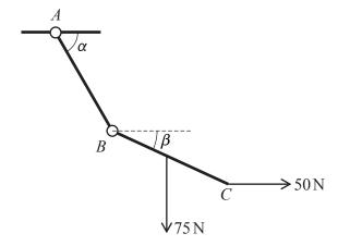
Two uniform rods AB and BC, each of length 2L, are freely jointed at B, and AB is freely jointed to a fixed point at A. The rods are held in equilibrium in a vertical plane by a light horizontal string attached at C. The rods AB and BC make angles  $\alpha$  and  $\beta$  to the horizontal respectively. The weight of rod BC is 75 N, and the tension in the string is 50 N (see diagram).
